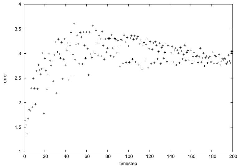
**Figure 4.7:** Error value distribution (reimplemented). The error signal is calculated by equation 3.7 on page 25 as in figure 4.6 on the preceding page. The error signal does not converge to 0, but to 3.
