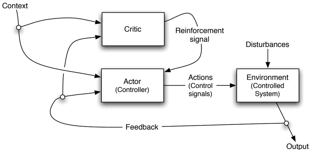
**Figure 2.2:** Actor-Critic architecture as a controller. The actor behaves as the controller in figure 2.1 on the facing page, acting on the environment to match the feedback with the contextual goal. The critic judges the actor by positive or negative reinforcement signals depending on the success of achieving the control objectives as provided by the context. Adapted from Barto (1995, fig. 1).
