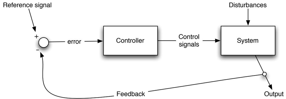
**Figure 2.1:** Negative feedback control system. The error is the difference between the reference signal and the output of the system. The difference is inputted to the controller which will issue control signals to modify the system as to minimise the error. Disturbances skew the system from the desired output. The desired output is fed to the controller as the reference signal.
